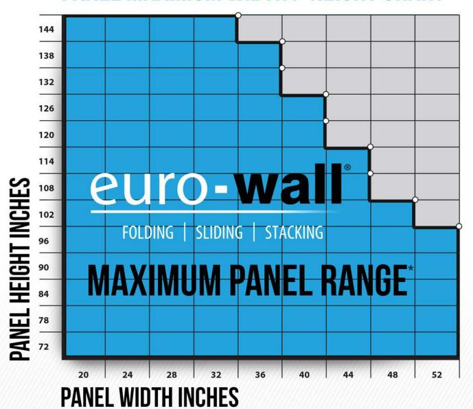
APPLIES TO BOTH INSWING AND OUTSWING CONFIGURATIONS, SEGMENTED AND RADIUS INSTALLATIONS.
